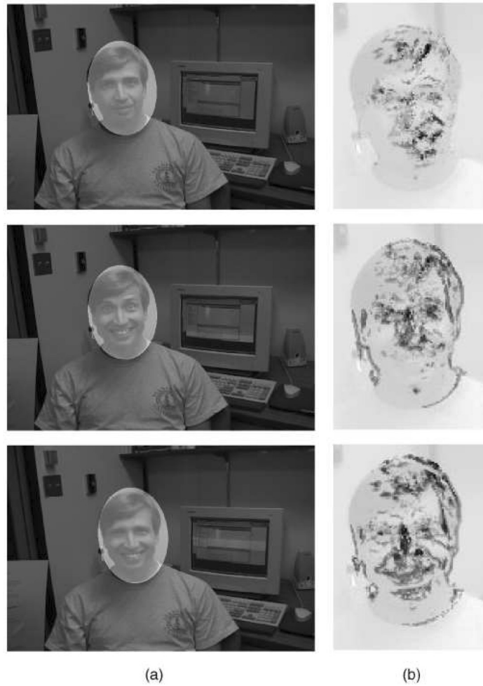
Fig. 13. Results of the robust online tracking method by Jepson et al. [2003] (a) The target region in different frames. (b) The mixing probability of the stable component. Note that the probabilities around the mouth and eyebrow regions change, while they remain the same in the other regions (©2003 IEEE).
